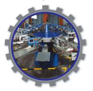
Plastisol, Glitter, Pigment and Foil Printing are some of the variants of screen printing. Azo-free dyes and chemicals are used and the customized prints in eye-catching colours leave a durable impression on the finished garments. The Printing Unit is equipped appropriately to produce 26,000 pieces per day and up to 20 colors in one design with automatic M&R machines.
